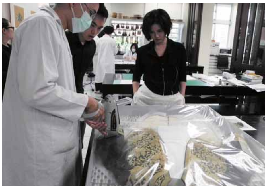
針對藏品進行 XRF 機械—金屬元素分析 The staff conducted a metal analysis of the artifacts with an XRF analyzer.
